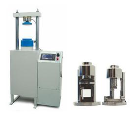
the required oil to the load frames for loading. Very silent power pack can load the specimen between 50 N/sec to 2.4 kN/sec with an accuracy of ±5%. A Rapid approach pump is supplied as standard. Safety valve (maximum pressure valve) is used to avoid machine overloading.
